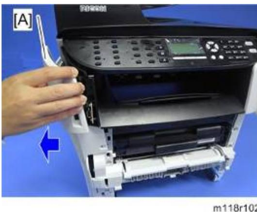
3. Pull the front upper part [A] of the left cover to release the hooks.
