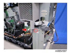
6. Remove the screw and disconnect the connector.
