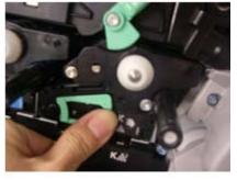
6. Check the pentagon-shaped window for all four colors. If you can see a red area, as shown in the "Incorrect" photo below, this means the unit was not *installed* correctly.
