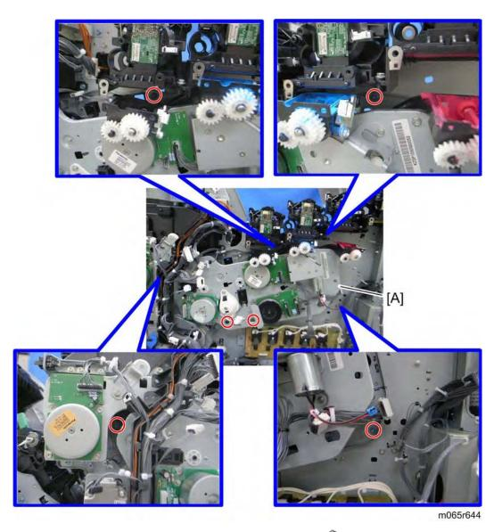
19. Gear unit [A] with the toner supply tubes for M, C and K ( x 6).
